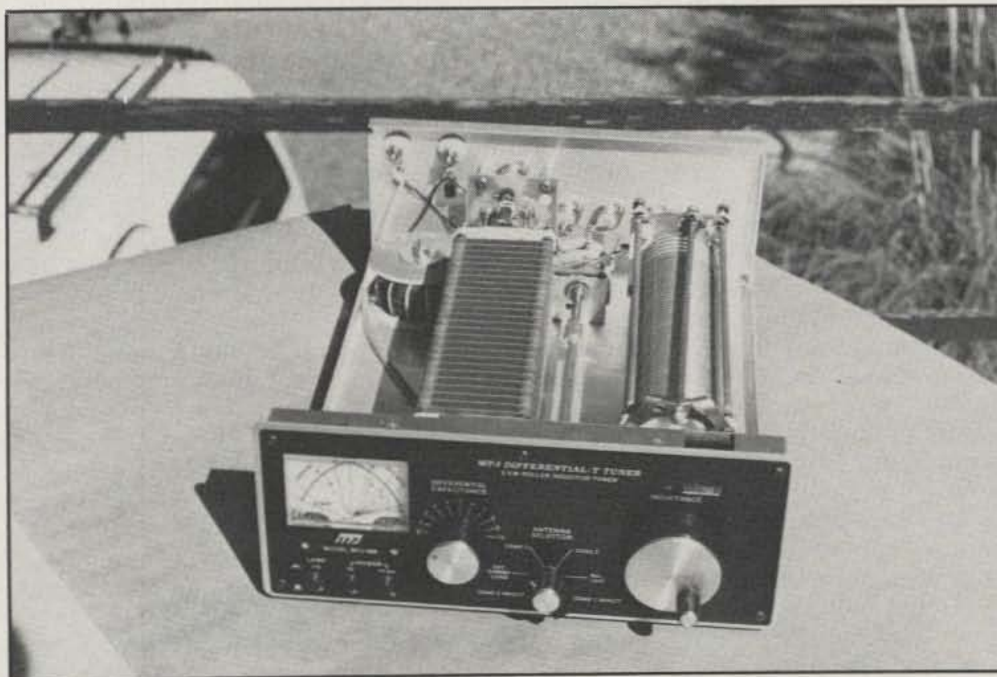
MFJ's differential capacitor Transmatch. This legal-limit unit does an outstanding job with both coax or tuned feeders.
